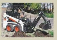
Backhoe Converts loader into a digging machine. Digging depths up to 5.5 ft.
